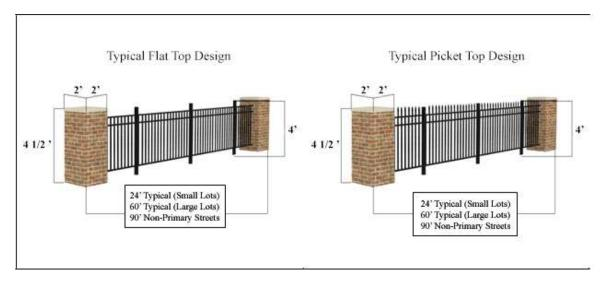
The fences shall be clear of signage or other obstructions. The specifications for the fencing are as follows:
