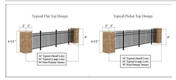
The fences shall be clear of signage or other obstructions. The specifications for the fencing are as follows:
