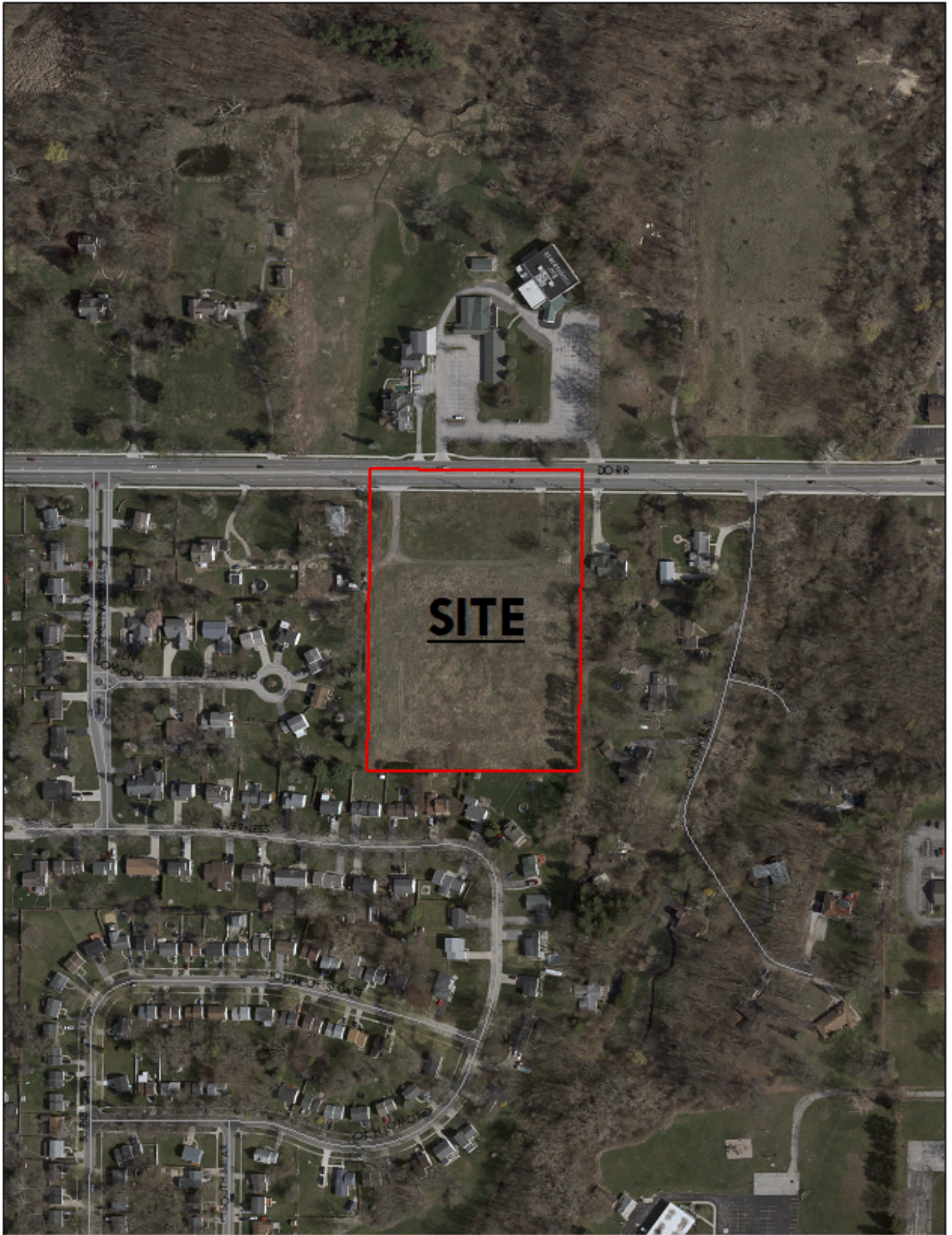
Aerial image of the property. The proposal is to develop a 32-lot duplex subdivision with a U-shaped Road connecting to Dorr Street at both ends.
