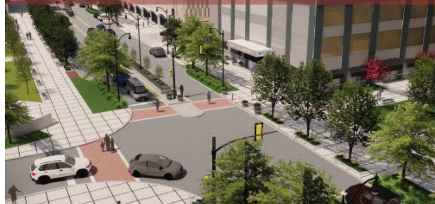
Alternative 1 – Reduce from Five (5) Lanes to Three (3) Lanes; Add On-Street Parking; Add Streetscape Improvements; Add Mid-Block Island
