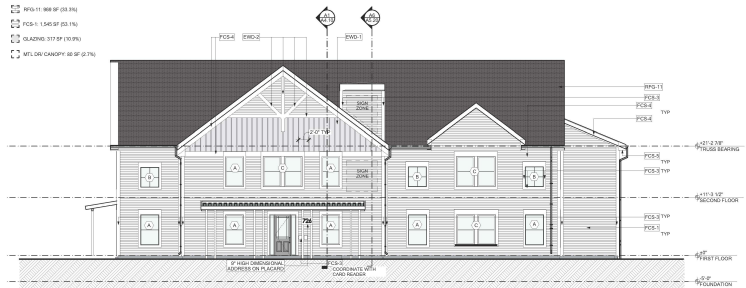
E1 WEST EXTERIOR ELEVATION SCALE: 1/8" = 1'-0"
