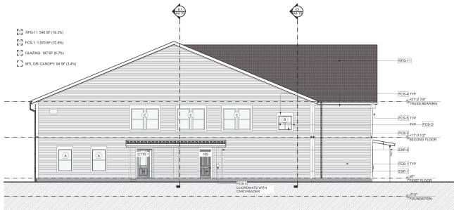
C3 NORTH EXTERIOR ELEVATION SCALE: 1/8" = 1'-0"
