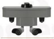
2 Fixed Axis 4MP HD Cameras each with 130° field of view (260° of visibility) with 2x Axis Q1700 License Plate Recognition Cameras
